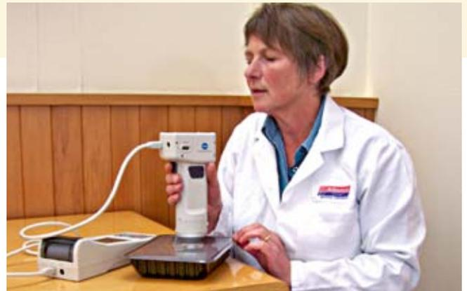
Figure 3. Colour stability measurement with a chromameter
