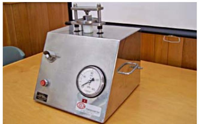
Figure 4. MIRINZ pneumatic tenderometer
